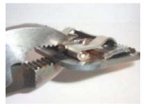
Bend until the flat part of socket is parallel with bottom of blade
