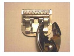
To fix the socket ears if they are too far in, get your pliers and set them to grab wide stuff. Put one part of the pliers on the outside edge of the blade, and the other part against the socket ear as shown in the picture on the left. Squeeze very gently so the ear is bent so it is perfectly vertical. Do the same to the other side.
