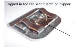
Another blade socket problem is where the socket part that fits over your clipper hinge is bent so it tips inward. This is caused by trying to force your blade on the clipper and it won't go on, thus bending the socket.
